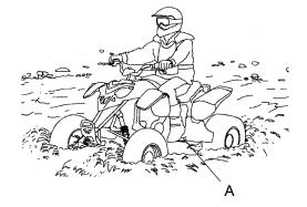
4. After driving through water, dry the brakes by applying light pressure to the levers until braking action is normal. If you do not perform this procedure, your brakes may be ineffective.
